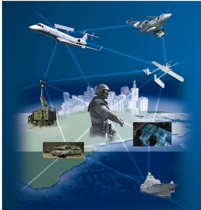
Figure 1: In the network-oriented defense concept decision makers, effectors, and information sources are interconnected in a common network. Functionality of a system is available as “services on the net”.
